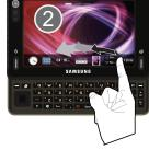
Note: Scrolling requires that you press firmly on the screen then drag. When scrolling through a list (see adjacent image) make sure not to touch or press individual entries on the list as this will open the list entry.
